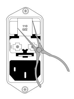
**3:** Use a small pair of needlenose pliers to gently pull out the mains jumper.
